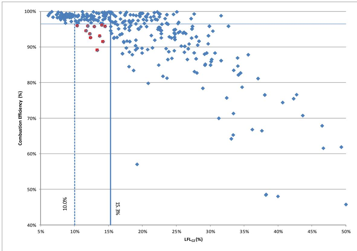
**Figure 3-3. Combustion Efficiency vs. LFL<sub>CZ</sub>**
